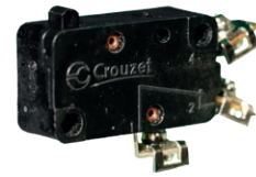
Customised version for nuclear application. Has radiation-resistant housing, 180 °C max operating temperature, W5 screw terminals and magnetic blowout for highly inductive circuit switching at 250 V ~
