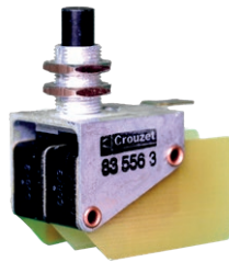
Telescopic plunger with Ø10 mm threaded barrel, metal bracket and plastic button. Single pole or double pole with staggered switchings (83556)
